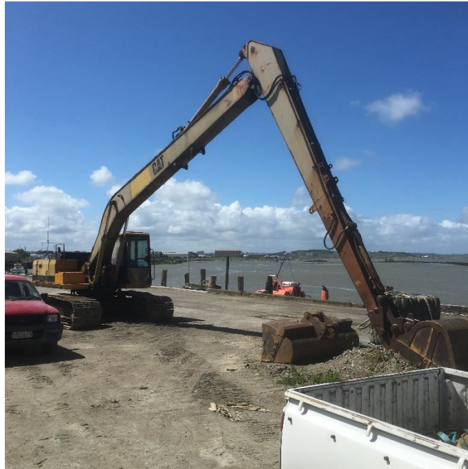
Long reach excavator for cargo and dredging work
